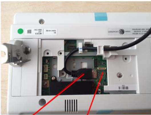
CABLE: OPERATION SUB-UNIT:USB3.0
