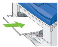
5 Slide both width guides until they rest lightly against the edge of the print media stack.
