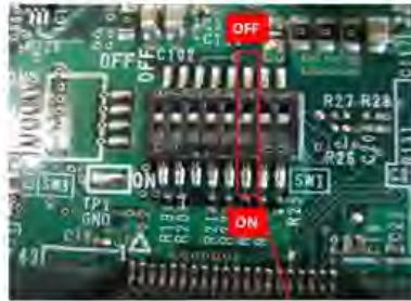
DipSW1-3 for CMOS CLEAR w_d238m1516a
